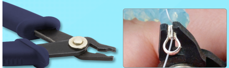
Use the EZ-Crimp Pliers (p. 99) to close EZ-Crimp Findings and Crimp Covers.
